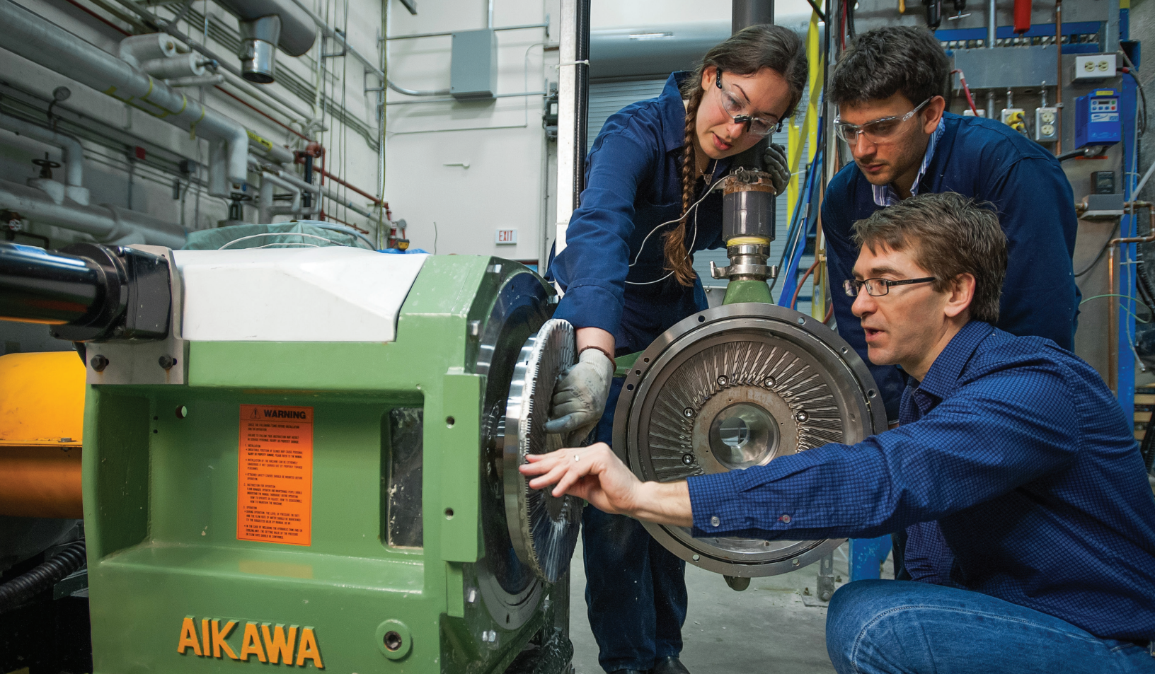
Above: James Olson, Francisco Fernandez and Nici Darychuk examine an experimental refiner plate on the PPC's low consistency refiner Photo: Martin Dee
